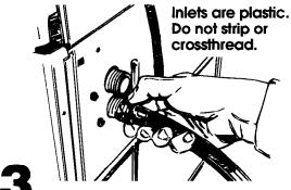
Attach hose (without adaptor) to bottom inlet valve opening first; then second hose (without adaptor) to top inlet. Tighten couplings by hand. Then use pliers to make an additional two-thirds turn.
